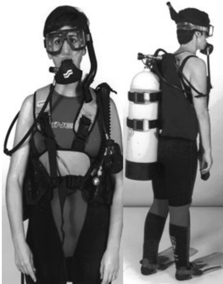
Figure 1. Front and side view of scuba diver equipped ready to jump into the water. She is carrying a compressed air tank, and is wearing a buoyancy compensator (BC), mask with snorkel, and fins. Her mouthpiece is attached to the second stage regulator, and it in turn is attached by hose to the first stage regulator on top of the tank. The alternate second stage regulator is shown over her left arm. Note: this diver is not wearing a weight belt; weights are carried inside her BC.
