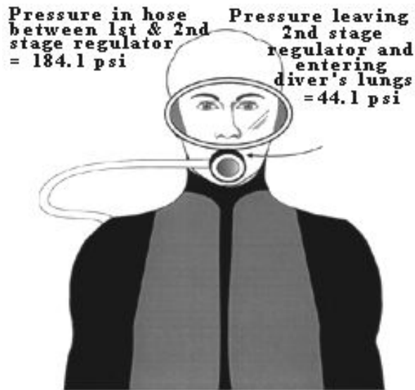
Figure 5. Scuba diver at 66 fsw (3 atm. or 44 psi) The pressure in the hose connecting the first stage and second stage regulators is the ambient pressure + 140 psi or 184.1 psi. The air pressure leaving her second stage regulator is at ambient pressure (44 psi). The pressure in the tank (on her back, not shown) does not affect the regulator pressures (as long as the tank pressure is above some minimum value, usually the ambient pressure).
